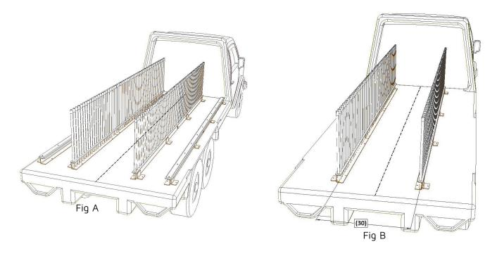
**Step 1**: Affix all eight mounting L brackets to the rack and bump rails using supplied 3/8" bolts, 5/16" flat washers, and 3/8" nyloc nuts (16 places).
